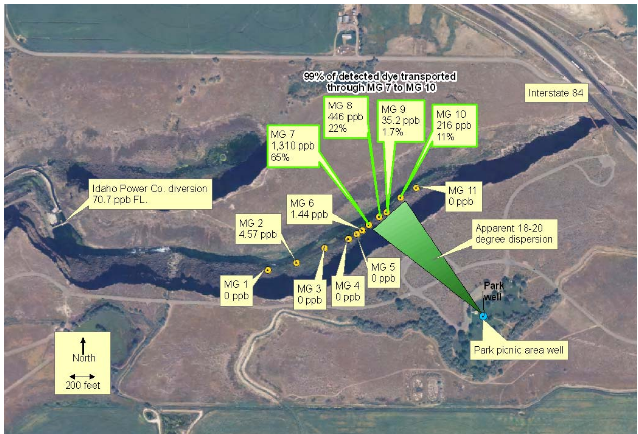
Figure 8. Air photo showing Fluorescein tracer test sample sites with yellow circles and the dye injection well in the Park picnic area with a blue circle. The majority of the detected Fluorescein dye passed by sites MG 7, 8, 9 and 10.
